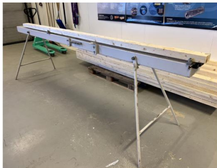
Figure. 4. Left: custom-built flatness reference table to quantify warp. Right: board distortion value “y” at 2 m length.
