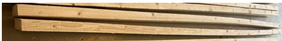
Figure 6. Boards from log 17. High bow rate in a green condition.
