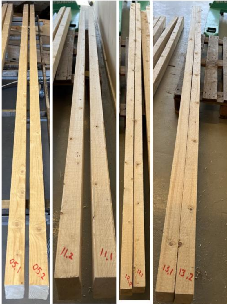
Figure 17.1. The boards with low bow and spring. The same boards as CT-scanned at Figure 17
