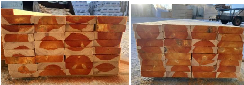
Fig. 2. B Mix(left) and Heartwood (right) batches pre-sorted at the sawmill, with heartwood reagent.
