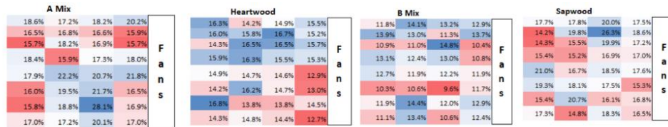
Fig. 6. Moisture content maps of 4 batches, kiln cross-section.
