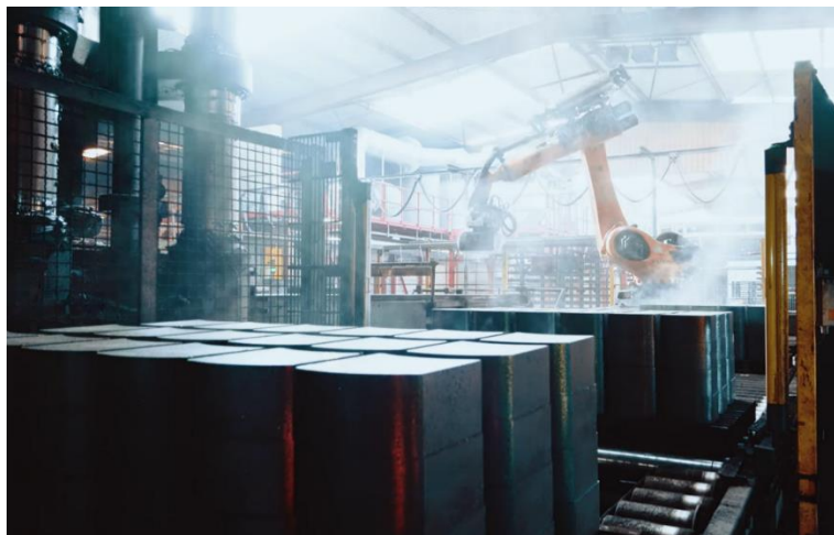
Figure 28. Intocast pressing process of hot pitch bonded paste in Oberhausen plant to produce magnesia-carbon bricks.
