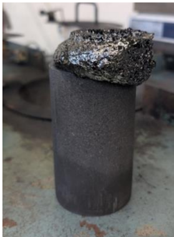
Figure 4. Foam-like SPL char, formed during TGA test.
