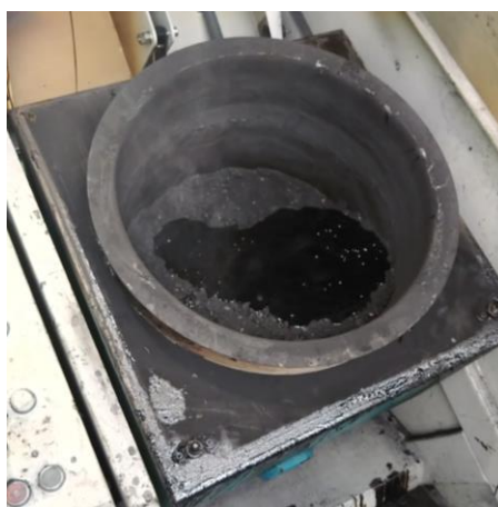
Figure 21. Preheated dry aggregate and molten binder inside the mixing bowl.
