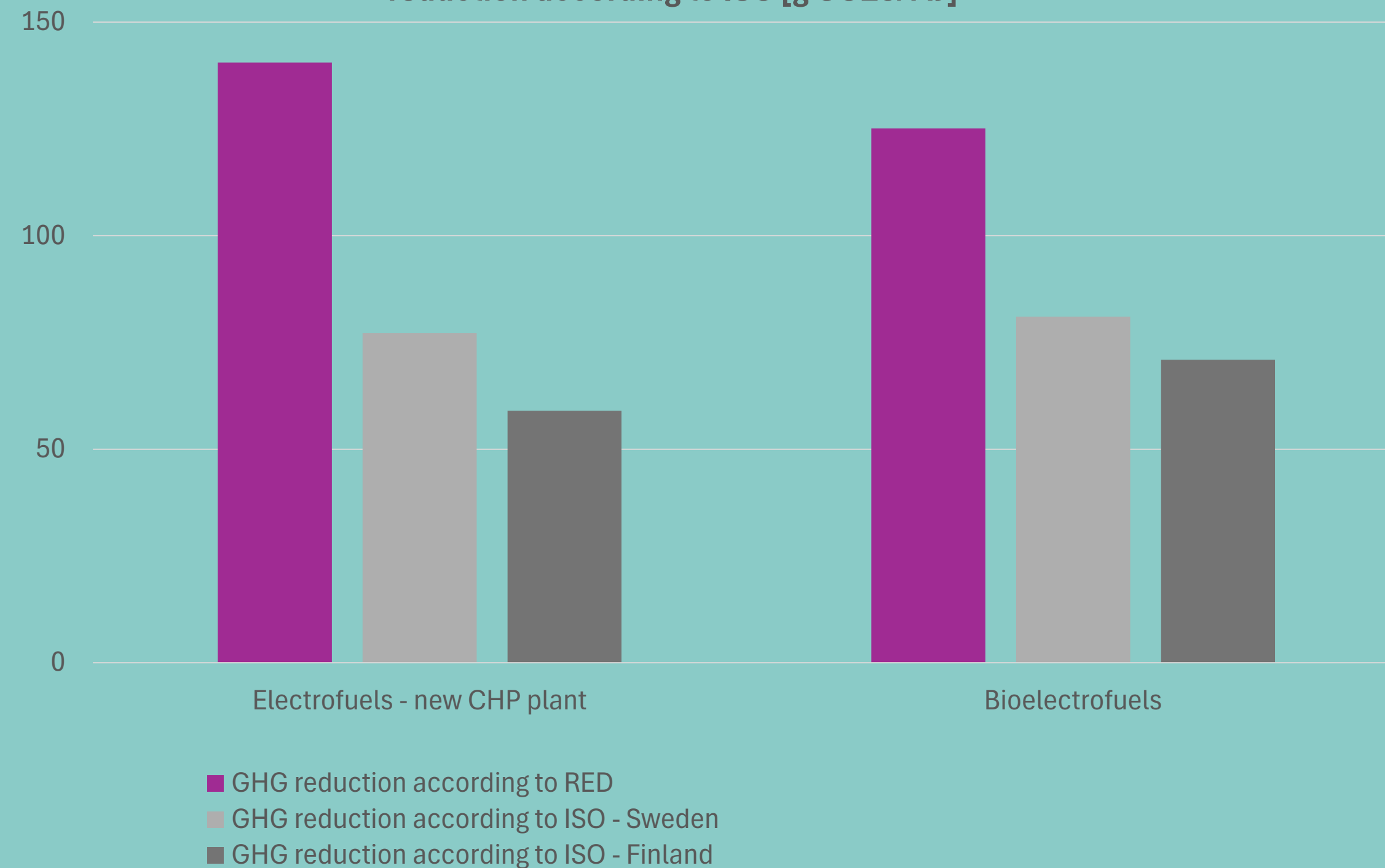
GHG reduction for use in shipping according to RED compared to GHG reduction according to ISO [g CO 2 e/MJ]
